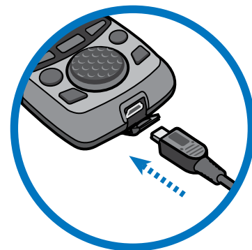
Fig. 3: Inserting the mini-USB connector
