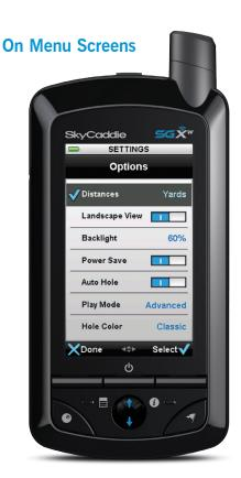
Slide your finger UP/DOWN to highlight the desired selection. Use the Left or Right Keys located directly beneath the display to make a selection.
