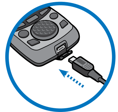
Fig. 3: Inserting the mini-USB connector
